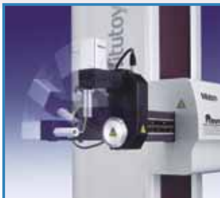
Position control of the holder-arm (vertical/horizontal)
