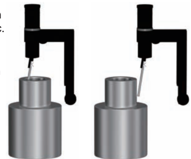
Making an inside-surface-related measurement / Making an outside-surface-related measurement
